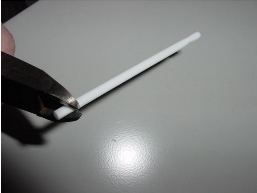
Figure 2a: Crimping the lollipop axle (Use just enough pressure to leave a mark: do NOT cut into the stick!)
