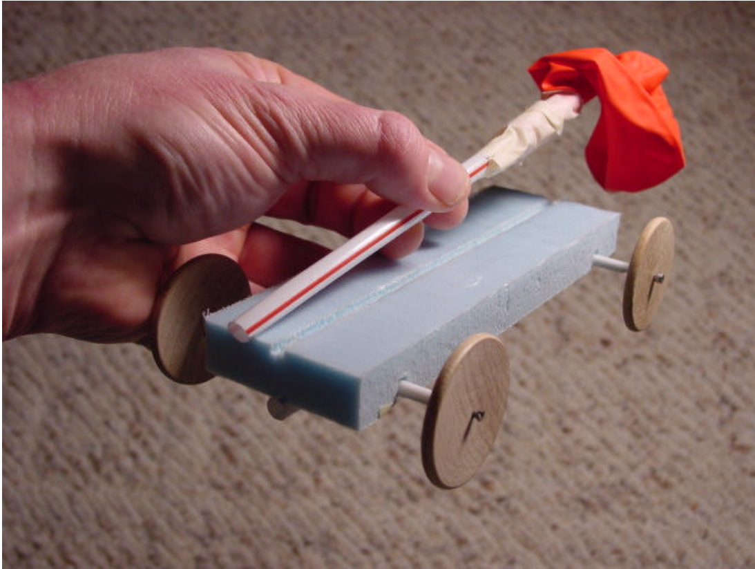
Figure 12: Aligning the straw with the lengthwise slot on the top of the car.
